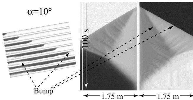
FIG. 14. Right: Spatiotemporal diagrams of the average concentration variations (gray levels) along the tube for  $\alpha=10^\circ$  with  $At=10^{-2}$ ,  $\nu=2 \times 10^{-6} \text{ m}^2/\text{s}$ ,  $d=20 \text{ mm}$  ( $Re_t \sin \alpha=80$ ). Vertical scale: time; horizontal scale: distance along the tube.—Left: sequence of views of the tube.
