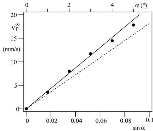
FIG. 10. Variation of the stationary front velocities as a function of  $\sin \alpha$  ( $At=3.9 \times 10^{-3}$ ,  $d=20$  mm, and  $\nu=10^{-6}$  m<sup>2</sup>/s). Black circles: experimental values estimated from the fits of Fig. 9. Dotted line: estimation of stationary front velocity assuming  $V_f^\infty = v_{\text{visc}}^\infty$  [Eq. (9)]. Continuous line: estimation from Eq. (35) derived theoretically in Sec. VII C.
