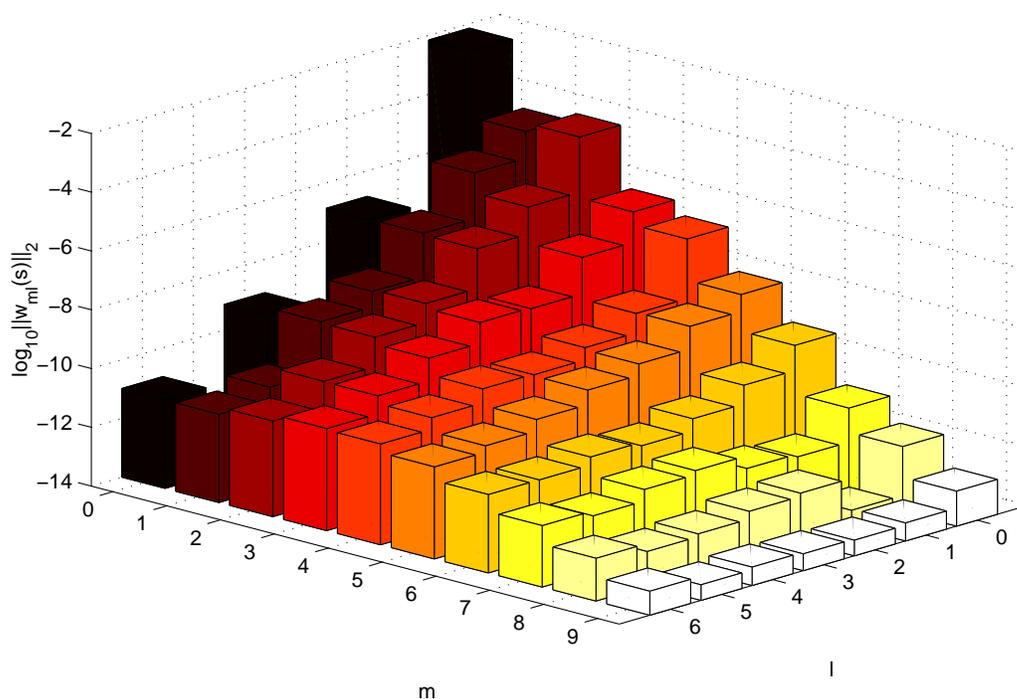
FIGURE 28. An example of the spectral energies ( $\|w_{ml}(s)\|_2 := \sqrt{\int_0^1 s|w_{ml}|^2 ds}$ ) in the axial and azimuthal spectral representation of the axial velocity for the  $\mathcal{R}_3$  travelling wave at its saddle node bifurcation for  $\alpha = 2.44$  (truncation (9,35,6)).
