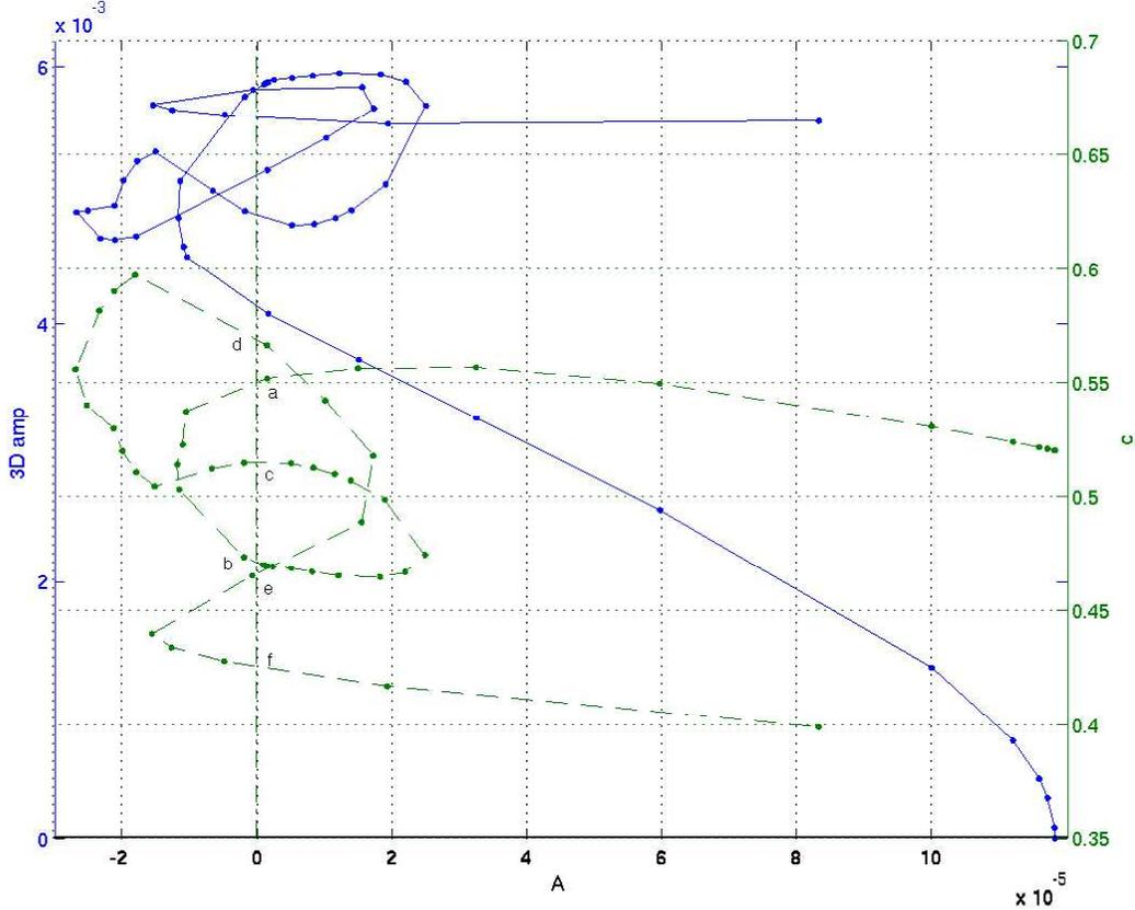
FIGURE 6. The continuation curve for  $m_0 = 3, \alpha = 2.44$  at  $Re = 2200$  ( $A_{crit} = 1.182 \times 10^{-4}$ , truncation (8,24,5)). Now we are sufficiently back from the saddle node bifurcation point to find more complicated behaviour. There are 6 crossings of  $A = 0$  indicating 6 travelling wave solutions at this  $\alpha$  and  $Re$  value! The various crossings have been labelled *a* through *f* for referencing in figures 7 and 8.
