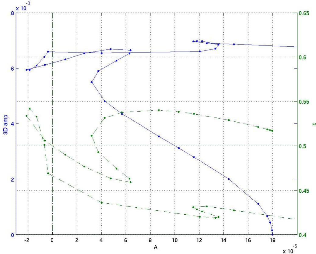
FIGURE 5. The continuation curve for  $m_0 = 3, \alpha = 2.44$  at  $Re = 1800$  ( $A_{crit} = 1.7962 \times 10^{-4}$  as opposed to  $A_{crit} = 1.75 \times 10^{-4}$  predicted from the SSP analysis: truncation (8,24,5)). Again there are two crossings of the pipe flow limit ( $A = 0$ ) representing an upper and lower branch of travelling wave solutions.
