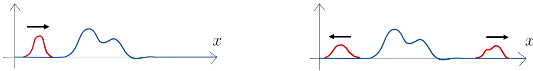
Figure 16. An intuitive idea of scattering, where an ingoing wavepacket (in red on the left) scatters off a potential (in blue) resulting into two outgoing wavepackets (in red on the right) is too hard!
